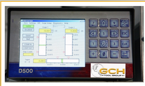
D500 controller for post-process gage unit
